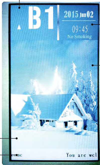
Real-time Elevator Status Display
